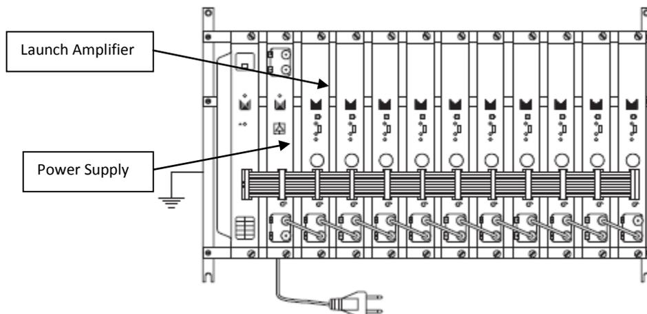
**IMPORTANT:** Layout of the modules must be as shown above. Power Supply (FA-310/312) must be located on the far left hand side and launch amplifier (PA-720) must be the next module in the chain. Please look at the above picture.
