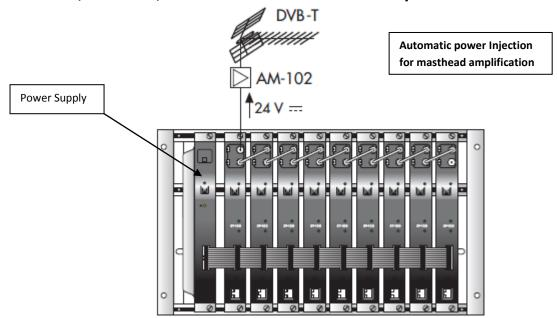
**IMPORTANT:** Layout of the modules must be as shown above. Power Supply (FA-310/312) must be located on the far left hand side and Terrestrial IP streamer must be the next module in the chain. Please look at the above picture.
