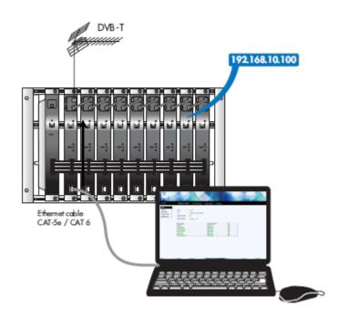
The picture above shows local mode configuration accessing each streamer individually and assigning new IP addresses. This is strongly advised prior to LAN network connection.
